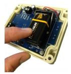
Insert the battery into the holder making sure the correct polarity of the connections, then push down at the base of the battery to secure in place.
