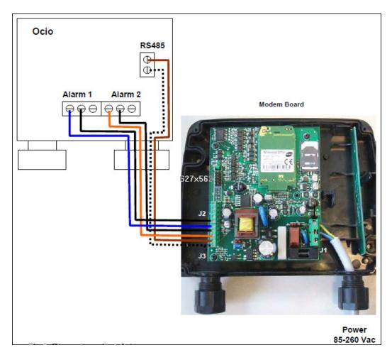
Carefully count the screw terminal connectors and wire them up as shown in the diagram.
