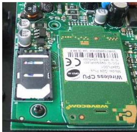
**Fig. 2:** Insert SIM Card.
