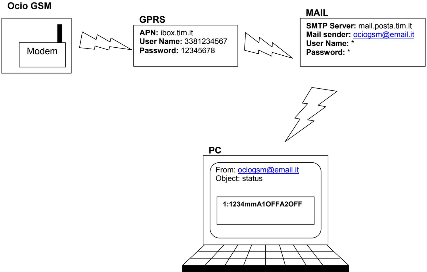
**Fig.13:** Sending email from the modem via GPRS.
