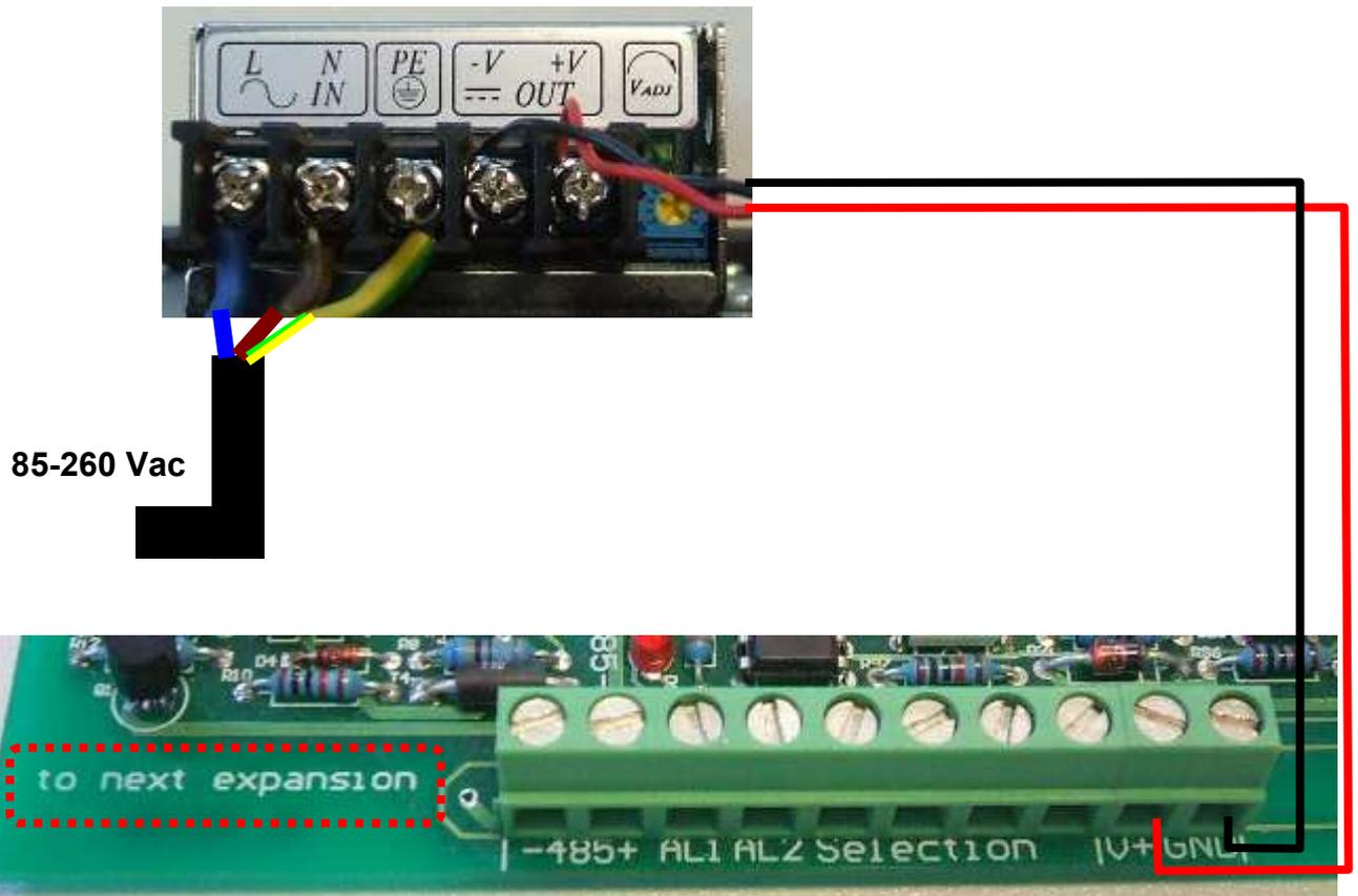
**Fig. 12:** Connection between Power Supply and expansion board
