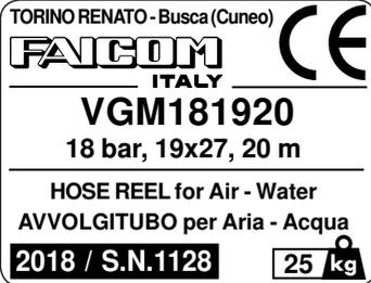
We affix the CE marking as the manufacturer of this equipment. On the equipment is securely attached a tag with curing adhesive system on which are indicated in addition to the name of the manufacturer and the symbol "CE", all information necessary for good identification of the machine (model, duty, year of construction, weight, etc.).
