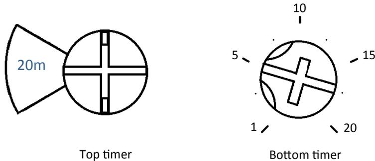
To adjust the timer (in minutes) the bottom timer can be set to the corresponding number, e.g. 1 is 1 minute and 15 is 15 minutes. The dial has mid-intervals which equate to 2.5 minutes, 7.5 minutes, 12.5 minutes and 17.5 minutes.
