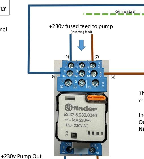
This circuit is for switching a 230v motor greater than 8A.
