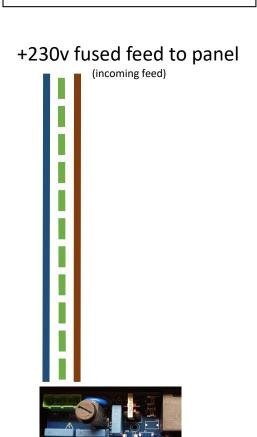
Connect the pump out power to the relay Coil **A1** = LIVE **A2** = NEUTRAL No Earth required for coil switching
