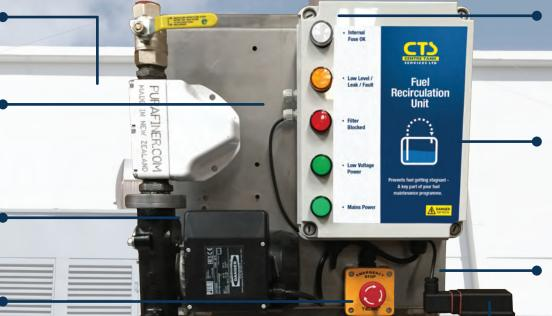
IP55 rated control panel with large, visible coloured lights for diagnosing any issues that need to be dealt with i.e. Filter blocked and low level/leak/fault.
