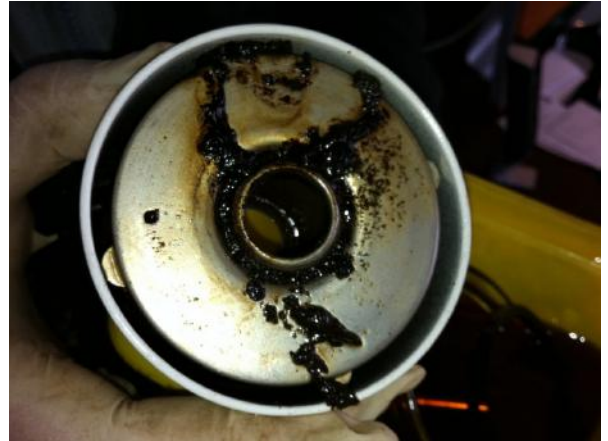
A filter clogged up with nasty diesel sludge
